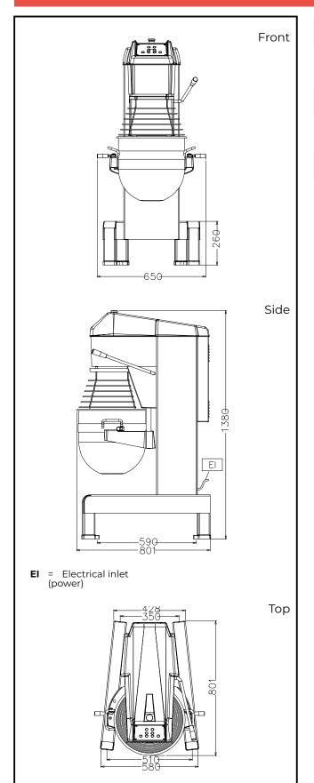
Electric Supply voltage: 600175 (DMBE40B) 200-240 V/1N ph/50/60 Hz 600176 (DMBE40B3) 380-480 V/3 ph/50/60 Hz Capacity: ISO 9001; ISO 14001 kg/ Performance (up to): Cycle 40 litres Capacity: Key Information: External dimensions, 655 mm Width: External dimensions, Depth: 850 mm External dimensions, 1370 mm Height: **Shipping weight:** 203 kg ISO 9001; ISO 14001 kg **Cold water paste:** with Spiral hook
